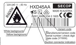
S = Static cooling normally sufficient
